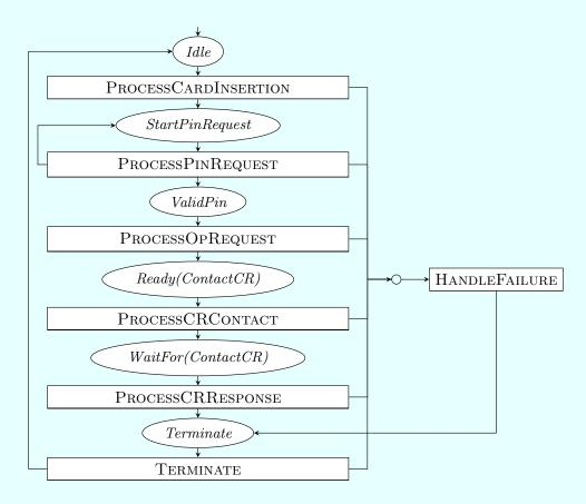
Component failure triggers exit to HANDLEFAILURE component.
